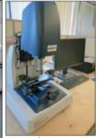
2014 Bruker Contour GT-K 3D Optical Microscope
