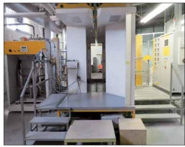
2008 ITW Gema Magic Compact BA02 10 Gun Powder Coat Paint System & GEMA PZ Powder Center Quick Color Change Module
