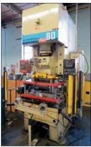
Comatsu OBS-80-VS-3 Gap Frame, 88 Ton, 37 – 75 SPM
