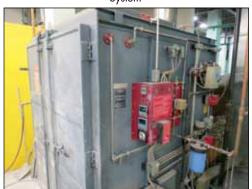
Controlled Pyrolysis Bake-Off Cleaning Furnace, Mdl. PRC 141 4140, 475,000 BTU
