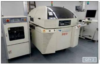
MPM Speedline UltraFlex 3000 Stencil Screen Printer
