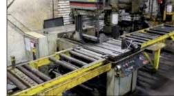
Marvel Vertical Band Saw Model 81/II, 18" x 20" Capacity
