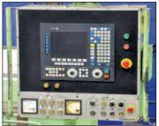
63"X 177" HEYLINGSTAEDT NDKB-1000/III CNC HEAVY DUTY LATHE, 63" Swing Over Bed, , 177.16" Between Centers, 48" 4-Jaw Chuck, 4-Position Turret, 2.8 – 560 RPM, 35,200 Lbs. Max. Capacity Between Centers (No Steady Rests), Fagor CNC Control, Retrofit 2009, 3-Way Bed, 9.84" Tailstock Quill Dia., 7.87" Quill Stroke, (2) Steady Rests, Chip Conveyor, 100 HP, S/N 000 932 34
