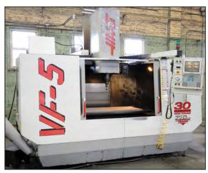
HAAS VF5 CNC vertical machining center
