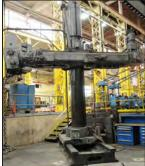
**KAUKAUNA** portable universal drilling, tapping & boring machine
