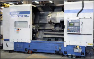
MORI SEIKI SL75MC CNC turning and live milling center
