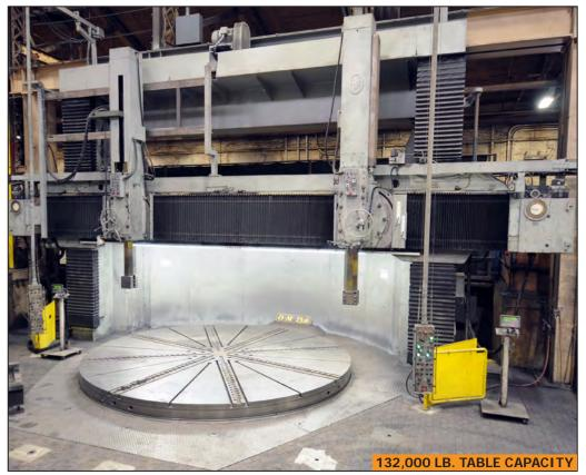
**O-M LTD.** TMD50/70 196.85"/275.59" vertical boring mill
