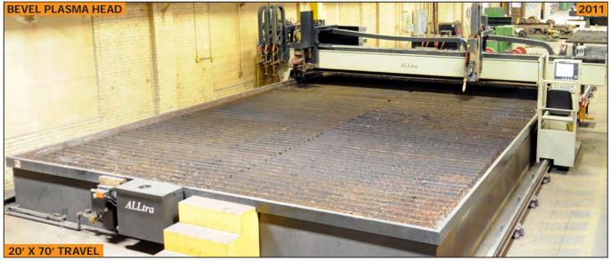
ALLTRA PG30-20S gantry type CNC shape cutting machine
