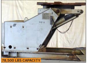
ESAB/PEMA 35000F tilt & rotate welding positioner
