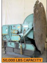
**ARONSON** GE500CS tilt & rotate positioner w/ geared elevation
