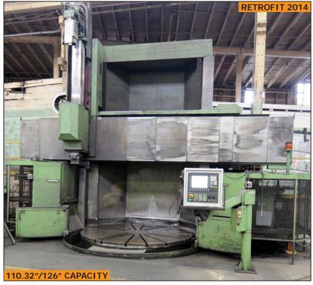
SCHIESS VERTIMASTER 32 DSC 280 CNC vertical turning, boring & live milling center
