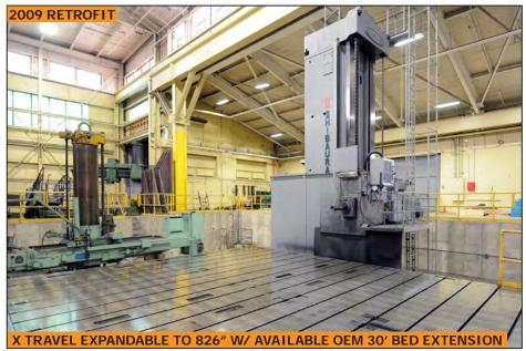
TOSHIBA/SHIBAURA BSF24/16 CNC 6.3" ram type horizontal boring mill
