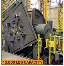
**WORTHINGTON** 400P tilt & rotate welding positioner
