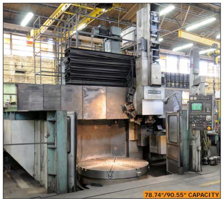
TOS SKS 20 CNC vertical turning, boring & live milling center
