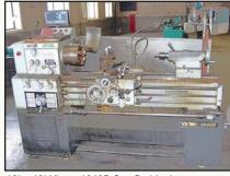
16" x 40" Victor 1640B Gap Bed Lathe
