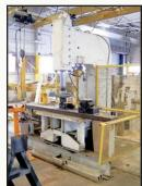
Hydraulic C-Frame Straightening Press
