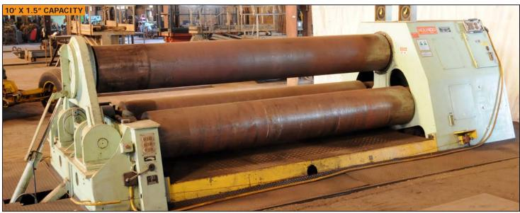
ROUNDO PS 460/10 hydraulic double pinch plate bending rolls
