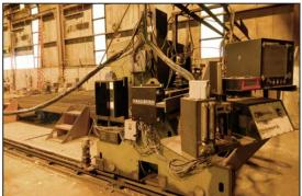
MG CUTTING SYSTEMS CNC plasma & oxy-acetylene cutting table
