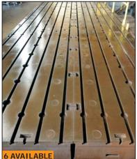
View of 138" x 69" x 14" T-slot floor plates
