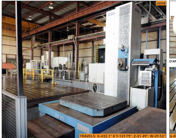
UNION P150/I, 5.9" CNC 7-axis floor type horizontal boring mill with in-feeding rotary table
