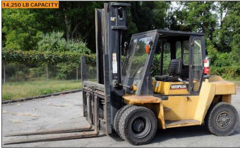
CATERPILLAR DP70 outdoor diesel forklift with cab enclosure
