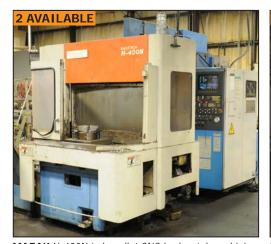
**MAZAK** H-400N twin pallet CNC horizontal machining center
