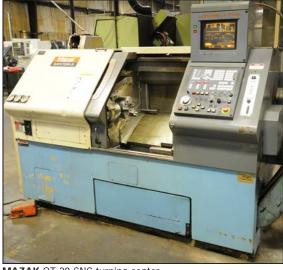
MAZAK QT 20 CNC turning center
