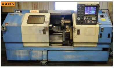
MAZAK QT 20N twin turret CNC turning center
