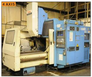
MAZAK AJV-25/405 bridge type CNC vertical machining center
