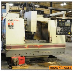
ZPS TREE VMC 1050/24 CNC vertical machining center
