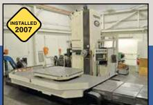
Toshiba Mdl. BP-130.R22 CNC Table-Type Horizontal Boring Mill
