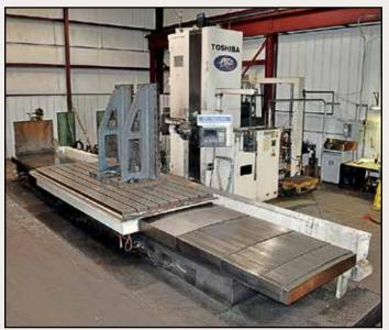
Toshiba Mdl. BP130-P40 CNC Table-Type Horizontal Boring Mill
