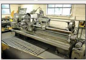
Lodge & Shipley AVS Mdl. 2013 20" x 78" Geared Head Engine Lathe
