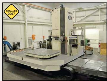
Toshiba Mdl. BP-130.R22 CNC Table-Type Horizontal Boring Mill
